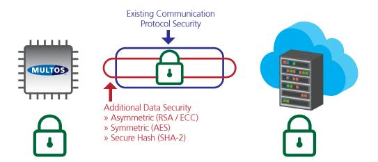
Symmetric or Asymmetric cryptography features can be employed to encrypt any data at risk, such that the data will be of no use to any third party accessing the data without authorisation.
