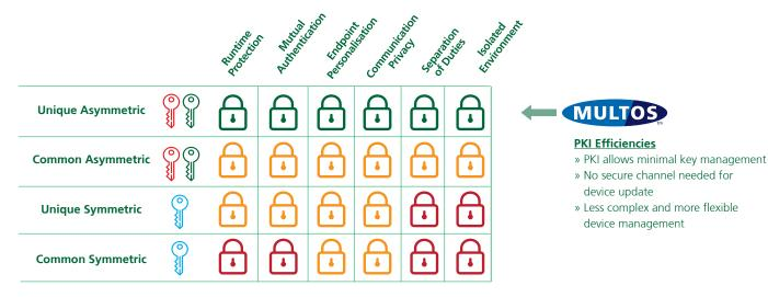
By using asymmetric cryptography, cost efficiencies could be realised, including:
